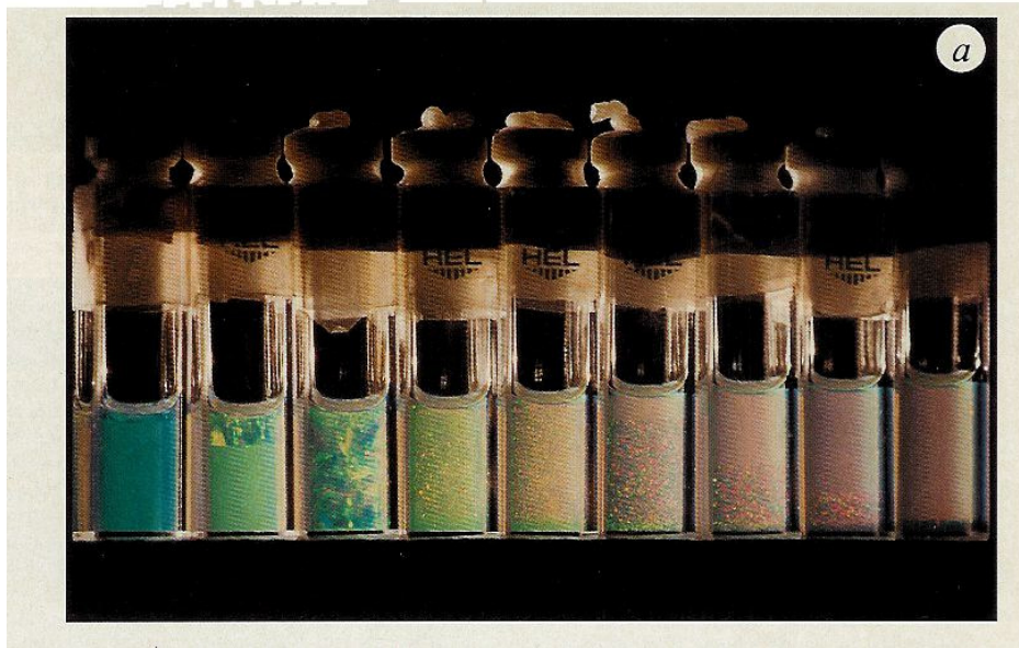
Figure 9.5: Refractive-index-matched suspensions of PMMA spheres of radius 325 nm illuminated by white light and photographed four days after shear-melting by tumbling. Concentration, in range 0.48 \leq \phi \leq 0.63 , increases from right to left and samples are designated by labels 2-10 (see fig. 9.6). Sample 2 is colloidal fluid. Samples 3-5 show coexisting fluid and homogeneously-nucleated polycrystalline phases. Samples 6 and 7 are fully polycrystalline. In samples 8-10 crystallisation is heterogeneously-nucleated. Lower portions of samples 9 and 10 remained amorphous (or glassy) for many weeks. From Pusey and van Meegen.
