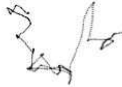
Figure 10.4: This plot shows about 30 s in the life of one Escherichia coli K-12 bacterium swimming in an isotropic homogenous medium. 18 The track spans about 0.1 mm, left to right. The plot shows 26 runs and tumbles, the longest run (nearly vertical) lasting 3.6 s. The mean speed is about 21 \mu\text{m/s} . From Berg H. C. Physics Today Jan 24 (2000).
